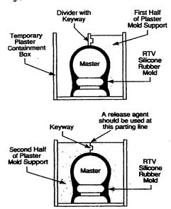
3. The master can now be removed to yield the finished mold.
