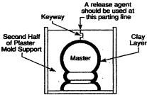
3. The hardened mold support is removed and then the layer of clay is removed.
