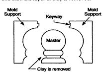
The master is now suspended in the inverted mold support leaving clear the area where the clay had been to provide a cavity.
