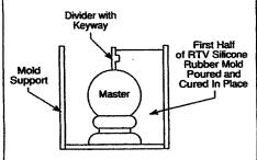
Remove the divider. Apply a mold release on the exposed portions of the first half of the mold which will contact the second half to prevent the two mold halves from adhering together. Pour the second half of the RTV silicone rubber mold and allow it to cure.
