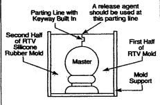
3. A cover is placed over what had been the top of the support where the RTV silicone rubber had been poured in. What had been the bottom is removed. This exposes the base of the master. The mold can be removed from the mold support. The two halves can then be separated to remove the master. When reassembled without the master, the two halves form a finished mold.
